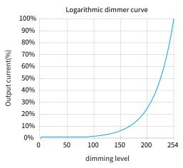
Remarks: The dimming curve can be selected by DALI configuration. The default is logarithmic dimming curve.
