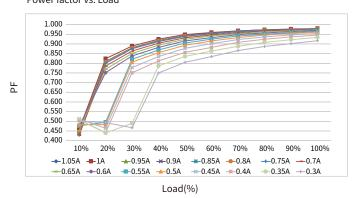
Displacement factor vs. Load
