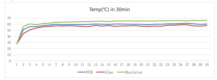
The above curves indicate the temp. changing in resistors, glue & PCB within 30 minutes after powering on, under the ambient temperature of 25  $^{\circ}$ C.
