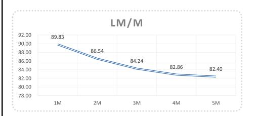
From above chart, please connect 5M at most by one-end power to keep brightness consistency.
